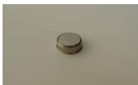
Figure 5. iButton data logger found on the Stryker X8000
